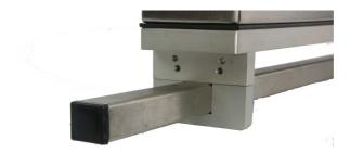
The 32mm diameter brackets allow 10mm of perpendicular movement which is useful for fine adjustment of Traverser position. Slots are provided in the brackets to accept locking rings (Domino Part No 5-0161129) these give additional anti-rotation support.
