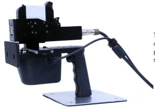
The Traverser cycle is initiated by pressing the trigger button on the handle. When triggered, the Traverser will move the printhead across the object to be printed and issue a print signal to the connected printer
